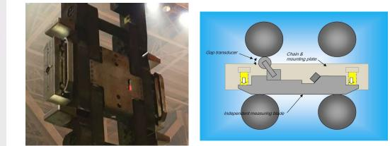
In-chain device gives reduced set of measurements at start of every sequence Use in combination with full gap head
