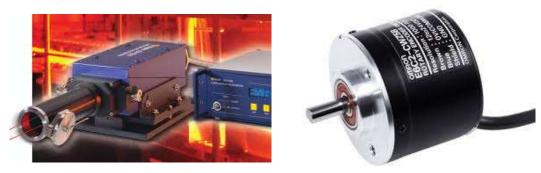
BFI Speed measurements can be made using laser velocimeters or encoders on non-driven rolls
