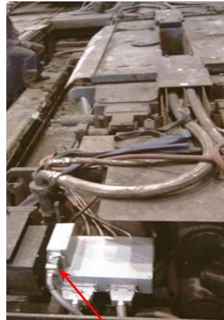
b) FOTS-connector and flexible optical cable
