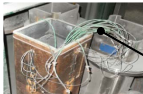
Cable bundle 15 thermocouple
