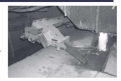
Powder application can be controlled using a variable rate feeder based on a model or equation taken from previous plant data. Feed rate is then set using casting parameters but must still be monitored and potentially adjusted by an operator.
