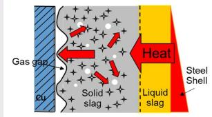
Fluoride-based phases (†) have been key to slowing shell cooling rate for best surface quality for peritectic steels In the second technique an increased number of iron particles are incorporated into the flux to reduce heat transfer without changing the flux composition.
