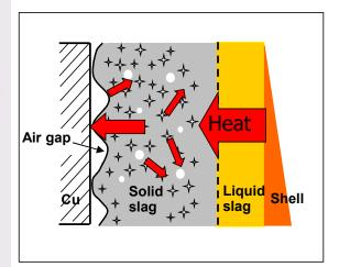
In **SLAGFILMOWL** the influence of basicity on crystallisation rate was shown and its impact on film thickness which in turn regulates the heat flux - the greater the degree of crystallisation the greater the film thickness.
