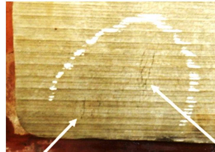
Near corner cracks Foot rolls or Zone 2. Two nozzles by billet face.
