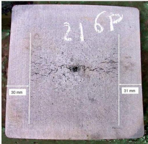
Half-way cracks Secondary cooling
