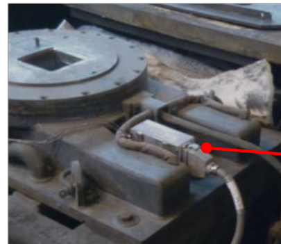
Instrumented mould ready for casting
